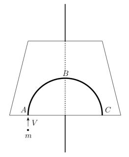
A heavy smooth lamina of mass M is free to slide without rotation along a straight line on a fixed smooth horizontal table. A smooth groove ABC is inscribed in the lamina, as indicated in the above diagram. The tangents to the groove at A and at B are parallel to the line. When the lamina is stationary, a particle of mass m (where m < M) enters the groove at A. The particle is travelling, with speed V, parallel to the line and in the plane of the lamina and table.
