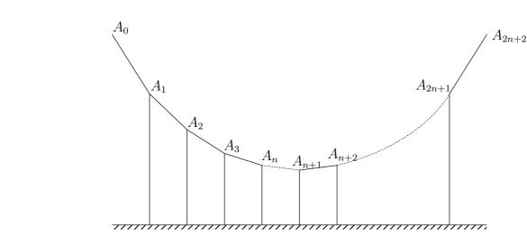
The above diagram represents a suspension bridge. A heavy uniform horizontal roadway is attached by vertical struts to a light flexible chain at points  $A_1 = (x_1, y_1)$ ,  $A_2 = (x_2, y_2), \ldots, A_{2n+1} = (x_{2n+1}, y_{2n+1})$ , where the coordinates are referred to horizontal and vertically upward axes Ox, Oy. The chain is fixed to external supports at points
