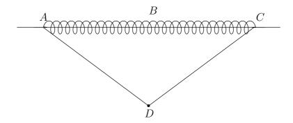
In the above diagram, ABC represents a light spring of natural length 2l and modulus of elasticity  $\lambda$ , which is coiled round a smooth fixed horizontal rod. B is the midpoint of AC. The two ends of a light inelastic string of length 2l are attached to the spring at A and C. A particle of mass m is fixed to the string at D, the midpoint of the string. The system can be in equilibrium with the angle CAD equal to  $\pi/6$ .
