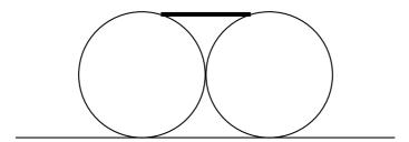
The coefficient of friction at all four contacts is  $\frac{1}{2}$ . The system is in equilibrium.
