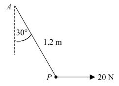
When a horizontal force of magnitude 20N is applied to P, it rests in equilibrium with the string making an angle of  $30^{\circ}$  with the vertical and AP = 1.2m as shown in Figure.
