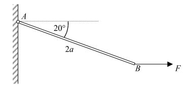
The rod is held in equilibrium inclined at an angle of  $20^{\circ}$  to the horizontal by a force of magnitude F newtons acting horizontally at B which is below the level of A as shown in Figure.
