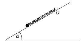
The particle is held at rest on the slope at a point 1.2m from O down the line of greatest slope of the plane.
