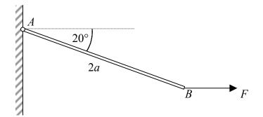
The rod is held in equilibrium inclined at an angle of  $20^{\circ}$  to the horizontal by a force of magnitude F newtons acting horizontally at B which is below the level of A as shown in Figure.
