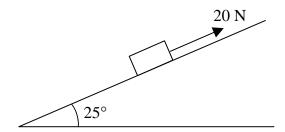
When the string is pulled with a force of 20N parallel to the line of greatest slope of the ramp, the lorry is on the point of moving up the ramp.
