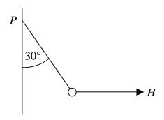
The other end is attached to a small object of weight 10N. The object is subjected to a horizontal force H so that the string makes an angle of  $30^{\circ}$  with the vertical.
