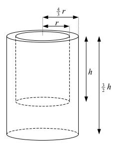
(a) Show that the centre of mass of the flask is a distance of  $\frac{9}{10}h$  from the open end of the flask. The flask is made from a material of density  $\rho$  and is filled to the level of the open plane face with a liquid of density  $k\rho$ . Given that the centre of mass of the flask and liquid together is a distance of  $\frac{15}{22}h$  from the open end of the flask,
