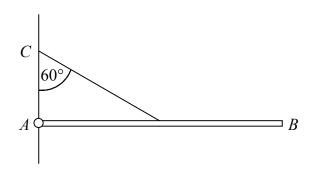
The end A is attached by a smooth hinge to a fixed point on a vertical wall so that the rod can rotate freely in a vertical plane. A mass of 6kg is placed at B and the rod is held in a horizontal position by a light string joining the midpoint of the rod to a point C on the wall, vertically above A. The string is inclined at an angle of  $60^{\circ}$  to the wall.
