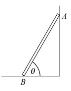
A man of mass 75kg ascends the ladder until he reaches a point P. The ladder is then on the point of slipping.
