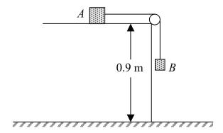
A light inextensible string of length 0.7m connects A to a particle B of mass 2kg. The string passes over a smooth pulley which is fixed to the edge of the table and B hangs vertically 0.4m below the pulley.
