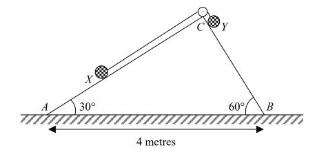
The two particles are connected by a light, inextensible string of length 2.5 metres passing over a smooth pulley at C which is the highest point of the two planes.
