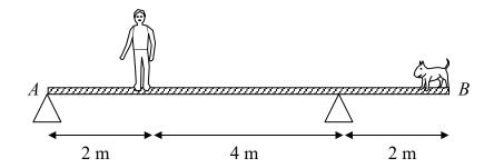
It is supported in a horizontal position by two pivots, one situated at A and the other 2 m from B. A man whose mass is 80 kg is standing on the plank 2 m from A when his dog steps onto the plank at B.
