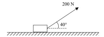
The tension in the rope is 200 N and it makes an angle of 40° with the horizontal. Under these conditions, the block is on the point of moving.
