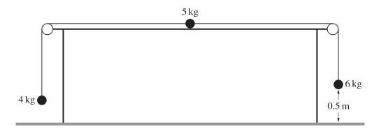
The diagram shows a particle of mass 5 kg on a rough horizontal table, and two light inextensible strings attached to it passing over smooth pulleys fixed at the edges of the table. Particles of masses 4 kg and 6 kg hang freely at the ends of the strings. The particle of mass 6 kg is 0.5 m above the ground. The system is in limiting equilibrium.
