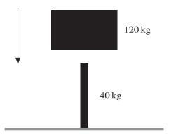
A metal post is driven vertically into the ground by dropping a heavy object onto it from above. The mass of the object is  $120\,\mathrm{kg}$  and the mass of the post is  $40\,\mathrm{kg}$  (see diagram). The object hits the post with speed  $8\,\mathrm{m\,s^{-1}}$  and remains in contact with it after the impact.
