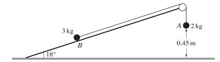
Two particles A and B of masses 2 kg and 3 kg respectively are connected by a light inextensible string. Particle B is on a smooth fixed plane which is at an angle of  $18^{\circ}$  to horizontal ground. The string passes over a fixed smooth pulley at the top of the plane. Particle A hangs vertically below the pulley and is 0.45 m above the ground (see diagram). The system is released from rest with the string taut. When A reaches the ground, the string breaks.
