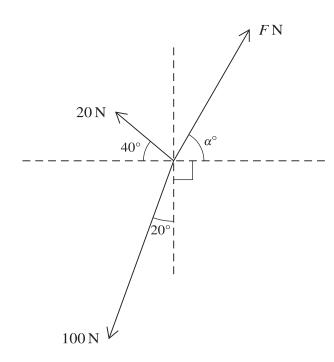
Three coplanar forces of magnitudes  $20\,\mathrm{N}$ ,  $100\,\mathrm{N}$  and  $F\,\mathrm{N}$  act at a point. The directions of these forces are shown in the diagram.
