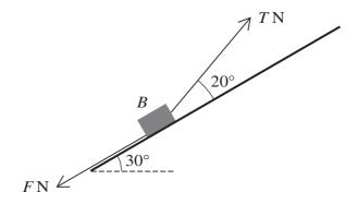
A block B, of mass 2 kg, lies on a rough inclined plane sloping at 30° to the horizontal. A light rope, inclined at an angle of 20° above a line of greatest slope, is attached to B. The tension in the rope is T N. There is a friction force of F N acting on B (see diagram). The coefficient of friction between B and the plane is  $\mu$ .
