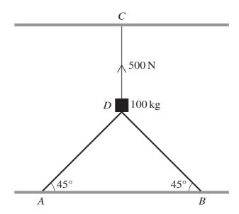
The diagram shows a block D of mass  $100\,\mathrm{kg}$  supported by two sloping struts AD and BD, each attached at an angle of  $45^\circ$  to fixed points A and B respectively on a horizontal floor. The block is also held in place by a vertical rope CD attached to a fixed point C on a horizontal ceiling. The tension in the rope CD is  $500\,\mathrm{N}$  and the block rests in equilibrium.
