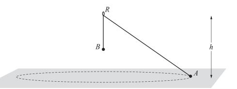
A light inextensible string is threaded through a fixed smooth ring R which is at a height h above a smooth horizontal surface. One end of the string is attached to a particle A of mass m. The other end of the string is attached to a particle B of mass  $\frac{6}{7}m$ . The particle B moves in a horizontal circle on the surface. The particle B hangs in equilibrium below the ring and above the surface (see diagram).
