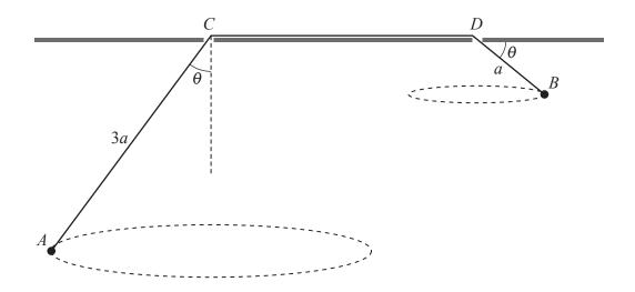
A light inextensible string AB passes through two small holes C and D in a smooth horizontal table where AC = 3a and DB = a. A particle of mass m is attached at the end A and moves in a horizontal circle with angular velocity  $\omega$ . A particle of mass  $\frac{3}{4}m$  is attached to the end B and moves in a horizontal circle with angular velocity  $k\omega$ . AC makes an angle  $\theta$  with the downward vertical and DB makes an angle  $\theta$  with the horizontal (see diagram).
