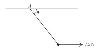
A particle of weight  $10\,\mathrm{N}$  is attached to one end of a light elastic string. The other end of the string is attached to a fixed point A on a horizontal ceiling. A horizontal force of  $7.5\,\mathrm{N}$  acts on the particle. In the equilibrium position, the string makes an angle  $\theta$  with the ceiling (see diagram). The string has natural length  $0.8\,\mathrm{m}$  and modulus of elasticity  $50\,\mathrm{N}$ .
