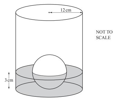
The diagram shows a cylinder containing water. There is a solid metal sphere touching the base of the cylinder. Half of the sphere is in the water.
